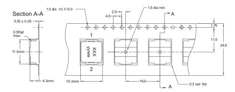
Supplied in tape-and-reel packaging, 950 parts per reel, 13" diameter reel.
